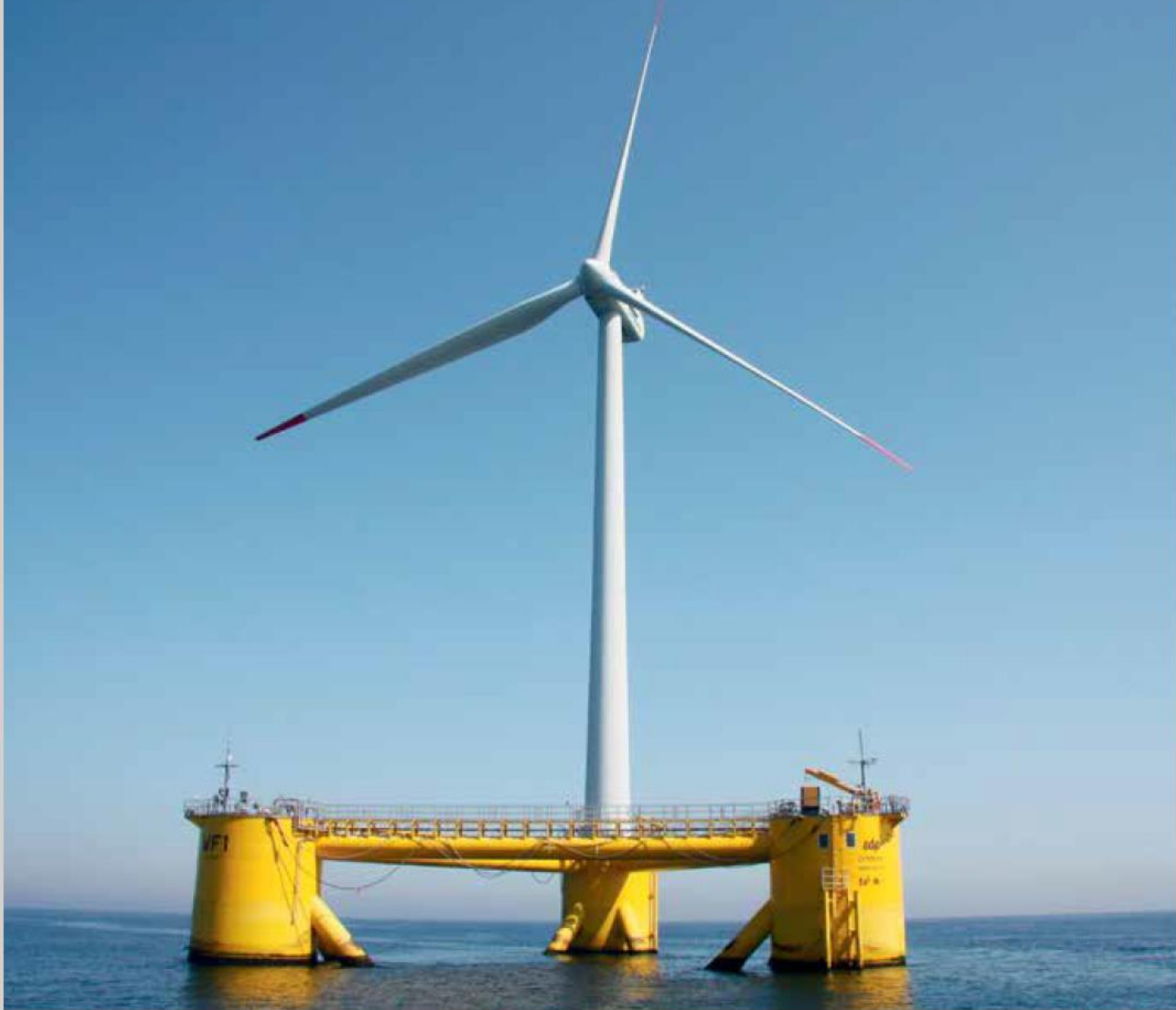
Floating offshore wind turbines (pictured) could unlock significant renewable energy capacity in the UK with low ecological risk, but research is needed to better understand impacts and identify appropriate sites.
