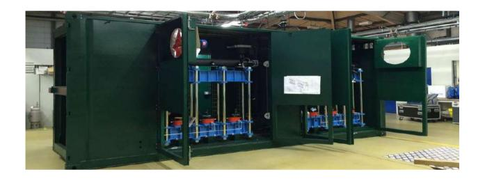
Surf & Turf CES / EMEC – Hydrogen fuel cell and electrolyser to explore off grid use of energy & local ferry use. Produced worlds first tidal powered hydrogen in 2017
