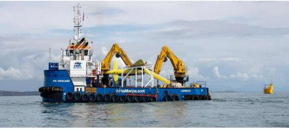
Minesto – Installed, commissioned and verified worlds first low speed tidal stream tech at commercial scale off Anglesey in N.Wales in 2018
