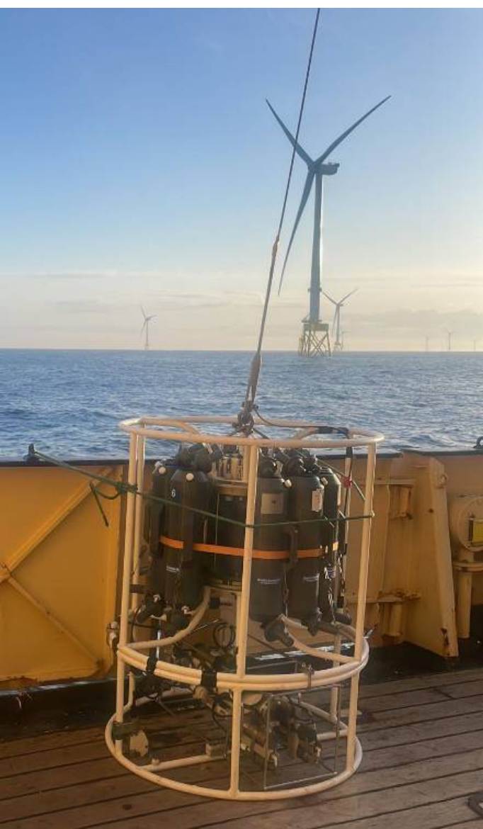
Fig. 3: CTD deployed in the vicinity of the Seagreen OWF
